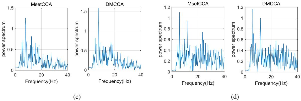
**Fig. 8.** Power spectra of test signals transformed by the reference templates extracted by DMCCA. The target frequencies are (a) 9.75, (b) 8.75, (c) 7.75 and (d) 5.75.
