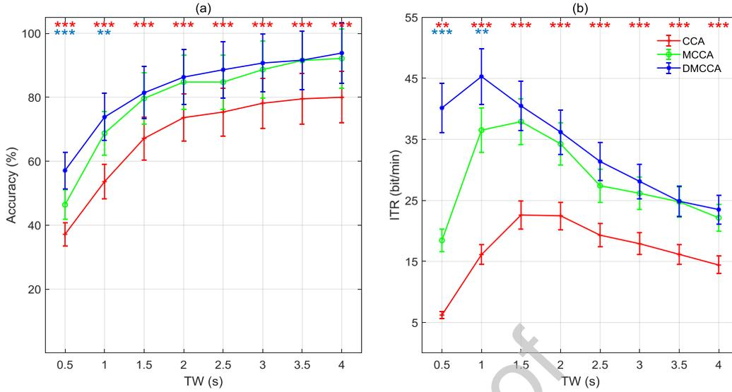
**Fig. 5.** Average accuracies of frequency recognition and information transfer rates (ITRs) of the 10 subjects derived by the CCA, MsetCCA, and DMCCA methods at various TWs ( $C = 8$ ). The significant difference between CCA, MsetCCA, and DMCCA methods obtained by one-way repeated measure ANOVAs is denoted by ‘\*\*\*’ (CCA:  $p < 0.001$ ), ‘\*\*’ (CCA:  $p < 0.01$ ), ‘\*’ (CCA:  $p < 0.05$ ), ‘\*\*\*’ (MsetCCA:  $p < 0.001$ ), ‘\*\*’ (MsetCCA:  $p < 0.01$ ), and ‘\*’ (MsetCCA:  $p < 0.05$ ).
