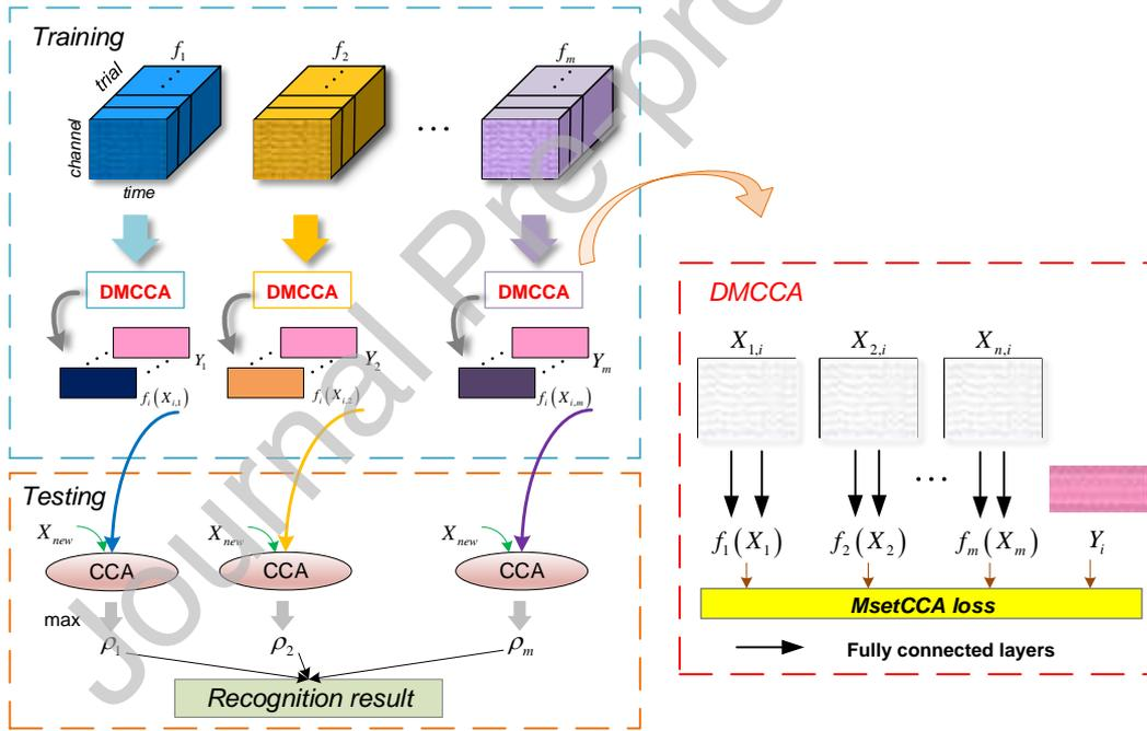
**Fig. 2.** Illustration of DMCCA-based method for SSVEP recognition.  $X_{i,j}$  is the EEG signals for the  $i$ th trial at the  $j$ th frequency, and  $Y_i$  is the reference signal at the  $i$ th stimulus frequency.  $X_{i,j}$  and  $Y_i$  are inserted into a DMCCA network to extract the most efficient features  $f(X_{i,j})$ . Recognition can be implemented among  $X_{new}$
