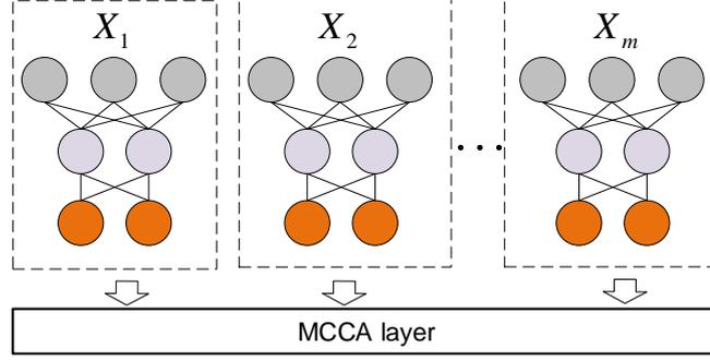
**Fig. 1.** Schematic of DMCCA. Multiple sets of variables  $\mathbf{X}_i$  are transformed by a group of fully connected neural networks. These NNs are optimized by the MsetCCA object, which maximizes the correlation of the output of these neural networks.
