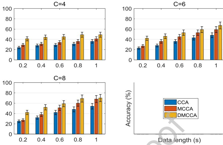
**Fig. 6.** Average SSVEP accuracies of the frequency recognition derived by the CCA, MsetCCA, and DMCCA methods under different channels ( $C = 4, 6, 8$ ) at TWs from 0.2 s to 1 s ( $C = 4$ : O1, O2, P3, and P4;  $C = 6$ : O1, O2, P3, P4, P7, and P8;  $C = 8$ : O1, Oz, O2 P3, P4, Pz, P7, and P8).
